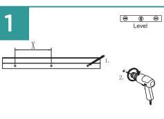
1. Level the hanging cleat with a level ruler and mark the installation hole position of the hanging cleat with a pencil. 2. Drill holes.
